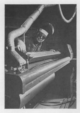
POSITIONING a cylinder on the automatic longitudinal welding machine, Leslie Cox completes setup operations. The machine automatically completes welding process.
